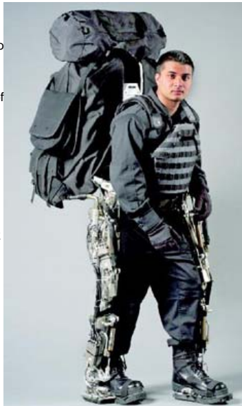
Bleex 1, an experimental exoskeleton, lets a person carry a 70-lb load, along with the 100-lb Bleex 1 itself, but feel as if he is carrying a 5-lb load.
