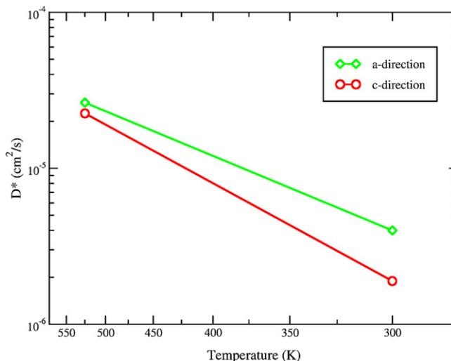
**Fig. 7.** Arrhenius plot of diffusivity with respect to temperature.
