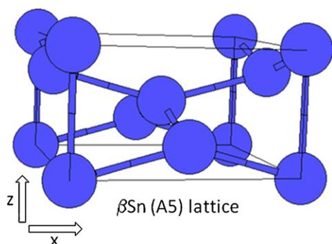
**Fig. 1.** Shown is the β-Sn (A5) lattice [28]. For the β-Sn phase, the tetragonal lattice constants used are  $a = 5.92 \text{ \AA}$  and  $c = 3.23 \text{ \AA}$ . 4 basis atoms are located at  $(0,0,0)$ ,  $(0.5,0,0.25)$ ,  $(0.5,0.5,0.5)$ ,  $(0,0.5,0.75)$  in lattice coordinates.
