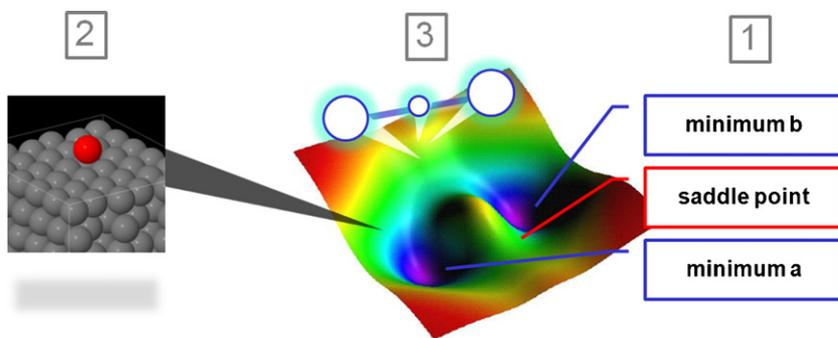
**Fig. 2.** (1) Typical locations on the energy hyper-surface for minima and saddle points. (2) An atomistic system represented by a point on the energy hyper-surface. (3) Multiple points (systems) with their distance in hyper-surface-space maintained.
