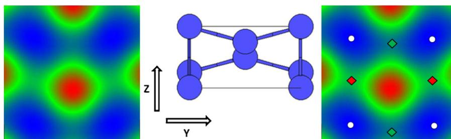
**Fig. 5.** Energy maps of the  $\beta$ -Sn (100) surface. (Left) Red denotes a higher energy (ion cores), blue denotes lower energy. (Right) Diamonds are respective saddle point locations of the adatom, white circles are minima locations.
