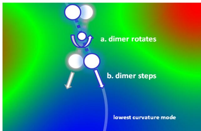
**Fig. 3.** When tracing the path of minimum energy from the saddle point to minimum, the dimer is rotated to a minimum energy via steepest descent (a) and then stepped (b), maintaining the correct orientation along the lowest curvature mode. This routine is repeated until the center of the dimer is at a minimum energy.
