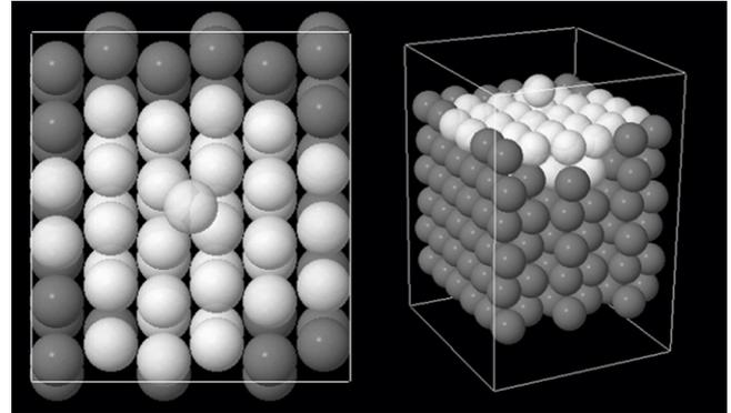
**Fig. 4.** (Left) A  $z$ -direction, top view of the (100) surface. (Right) A three-dimensional view of the simulation cell. Atoms are colored white to denote movable by the Dimer method and gray for fixed.
