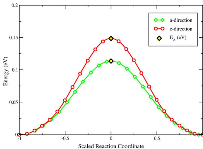
**Fig. 6.** Energy values along the minimum energy path for the given mechanisms. Values along the reaction coordinate are corrected to a baseline value of the minimum energy configuration—both mechanisms begin and finish at 0 eV. Diamonds denote energies corresponding to saddle point configurations.
